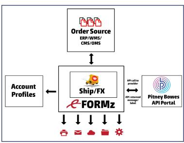
API keys are configured into the Ship/FX Account Profiles and connected utilizing the Secure Socket Layer (SSL) configuration through eFORMz. An API call to Pitney Bowes returns the label. eFORMz takes output from the WMS/ERP/OMS/CMS, formats it with the label and outputs it.
