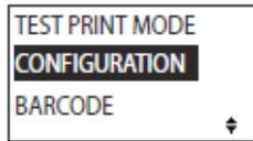
3. Press ENTER to go to the TEST PRINT SIZE. Select the print size with the arrow keys.
