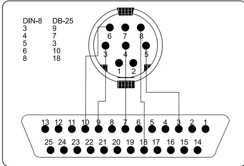
The above illustration shows a DIN-8 connector, front view (Mac), and a DB-25P connector, back view - solder side (HP).
