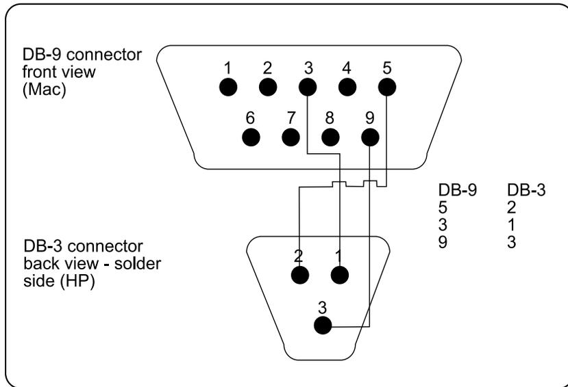
The above illustration shows a DB-9 connector, front view (Mac) and a DB-3 connector, back view - solder side (HP).
