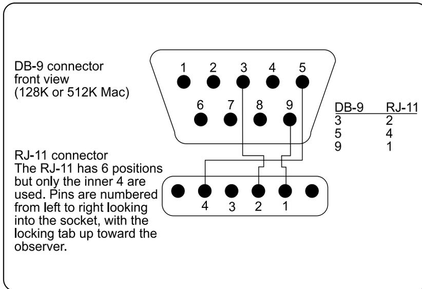
The above illustration shows a DB-9 connector, front view (128K or 512K Mac), and a RJ-11 connector. The RJ-11 has 6 positions but only the inner 4 are used. Pins are numbered from left to right looking into the socket, with the locking tab up toward the observer.
