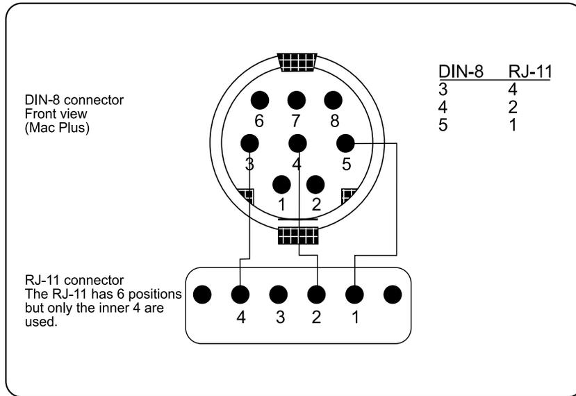
The above illustration shows a DIN-8 connector, front view (Mac Plus), and a RJ-11 connector. The RJ-11 has 6 positions but only the inner 4 are used. Pins are numbered from left to right looking into the socket, with the locking tab up toward the observer.
