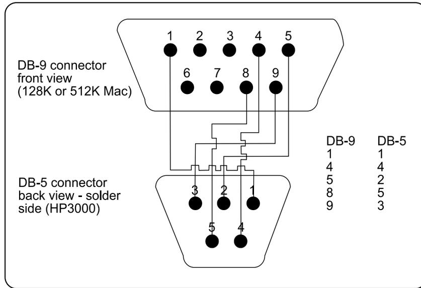
The above illustration shows a DB-9 connector, front view (128K or 512K Mac), and a DB-5 connector, back view - solder side (HP3000).
